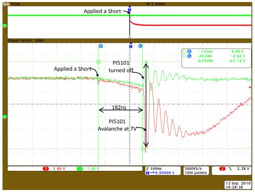
Test Setup: DUT: PI5101-EVAL1 Vin1 = 3.3V Vin2 = 3.3V Output Load = 20A
