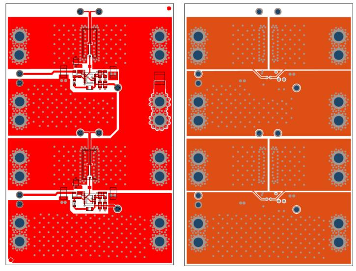
Figure 6: PI5101-EVAL1 layout top layer. Scale 2.0:1
