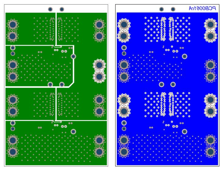
Figure 8: PI5101-EVAL1 layout mid layer 1. Scale 2.0:1
