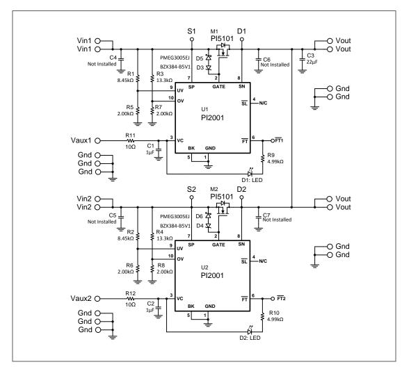
Figure 2: PI5101-EVAL1 Evaluation Board schematic.
