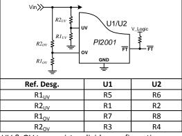
Figure 4: UV & OV two resistor divider configuration
