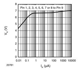
Fig. 5 - Typical Reverse Voltage V<sub>R</sub> vs. Reverse Current I<sub>R</sub>
