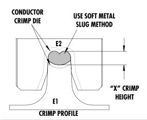
Use soft metal slug (solder) method to measure the "X" dimension. Verify tooling crimp height calibration by referring to the Go/No Go dimensions shown in the chart below.
