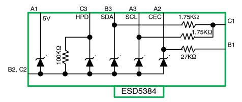
Figure 1. Electrical Schematic
