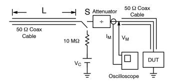
Figure 18. Simplified Schematic of a Typical TLP System
