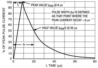
Figure 15. 8 x 20 μs Pulse Waveform
