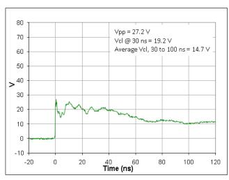
Figure 5. ESD Clamping Voltage Screenshot Positive 8 kV Contact per IEC61000-4-2, SCL line
