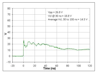
Figure 11. ESD Clamping Voltage Screenshot Positive 8 kV Contact per IEC61000-4-2, 5 V line
