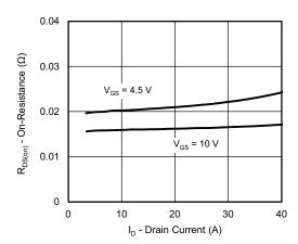
On-Resistance vs. Drain Current and Gate Voltage
