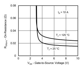
On-Resistance vs. Gate-to-Source Voltage
