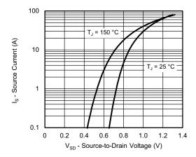
Source-Drain Diode Forward Voltage
