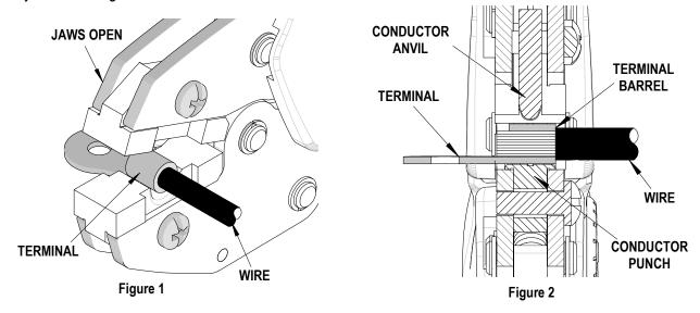
**Note**: Whenever crimping unbrazed product, make sure the seam of the terminal is oriented up or down in the tool. This will provide higher pull force values.
