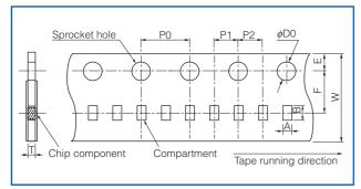
Embossed Carrier Taping EXC14C, 16C
