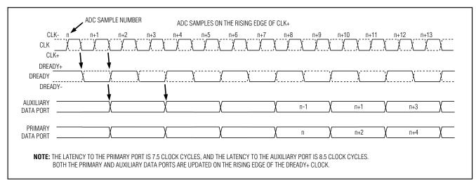
Figure 7. Demuxed DIV2-Mode Timing Diagram
