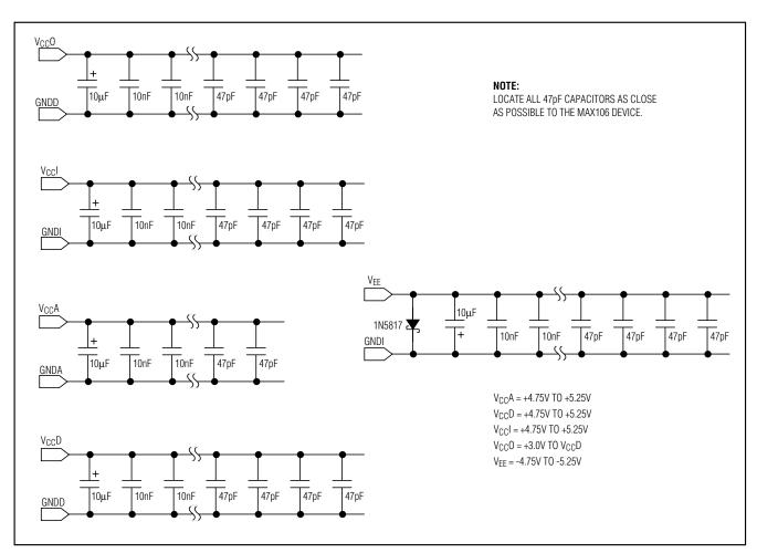
Figure 22. MAX106 Bypassing and Grounding
