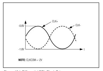
Figure 13d. Differential ECL Clock Drive
