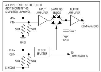
Figure 3. Internal Structure of the 2.2GHz T/H Amplifier
