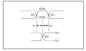
Figure 15. Reset Input Timing Definitions
