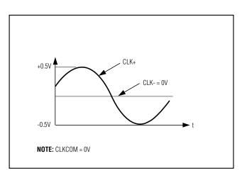
Figure 13a. Single-Ended Clock Input Signals
