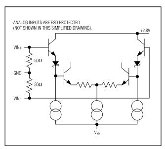
Figure 9. Simplified Analog Input Structure (Single-Ended/ Differential)
