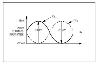
Figure 10b. Differential Analog Input Signals
