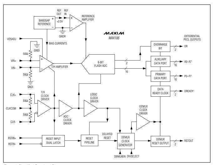
Figure 1. Simplified Functional Diagram
