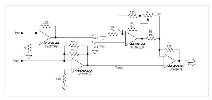
Figure 20. Die Temperature-Acquisition Circuit with the MAX479
