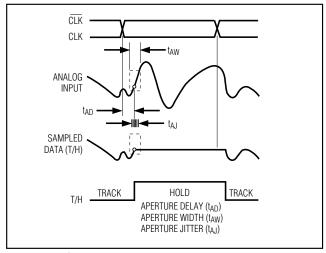
Figure 4. T/H Aperture Timing
