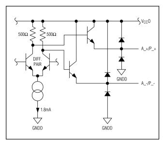
Figure 5. Simplified PECL Output Structure
