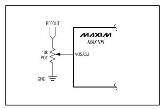
Figure 11. Offset Adjust with External 10k $\Omega$  Potentiometer
