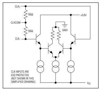
Figure 12. Simplified Clock Input Structure (Single-Ended/ Differential)
