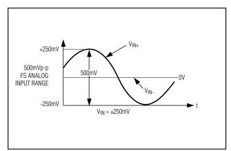
Figure 10a. Single-Ended Analog Input Signals
