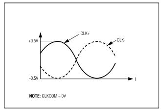
Figure 13b. Differential Clock Input Signals
