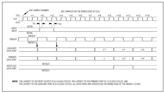
Figure 18. Reset Output Timing in Demuxed DIV2 Mode (DREADY Aligned)
