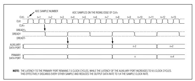
Figure 8. Decimation DIV4-Mode Timing Diagram
