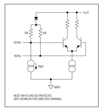
Figure 14. Simplified Reset Input Structure
