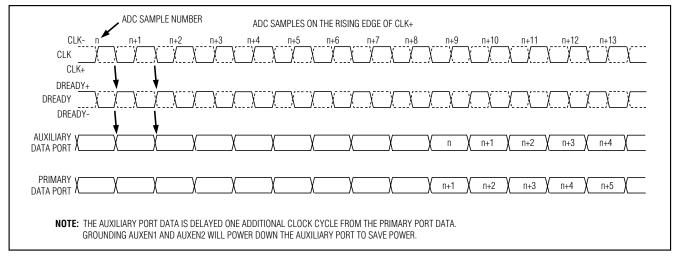
Figure 6. Non-Demuxed, DIV1-Mode Timing Diagram
