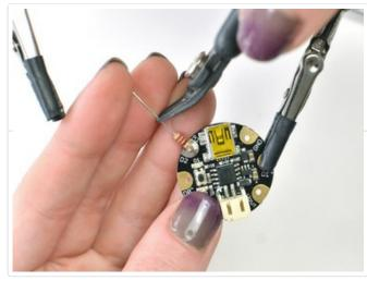
Next it's time to connect up the center leg of the transistor.
