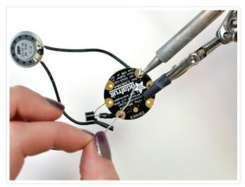
Tin the last remaining lead of the transistor and solder to a piece of wire. Slide on some heat shrink and use a heat gun to shrink it.
