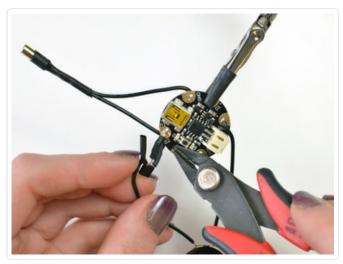
Your circuit is complete! Look it over, comparing it to the circuit diagram and double checking your solder joints.
