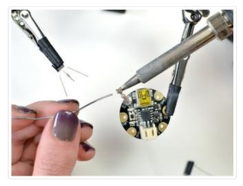
Don't forget heat shrink tubing! Cut a small piece of the medium size and place it over the resistor.
