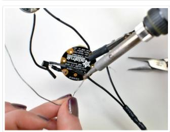
Solder the other end of the wire, along with one of the wire leads of the tilt ball switch, to GND on GEMMA.
