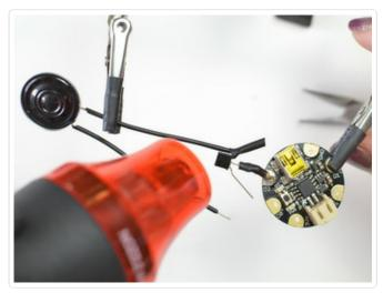
Bend the speaker's other wire to the Vout pin on GEMMA and solder in place.
