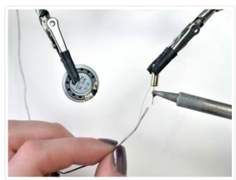
Hold a wire up to the speaker's pad and reheat the solder with your soldering iron. Hold it to the joint until the solder flows around the wire, then remove heat and hold the wire until the solder solidifies.
