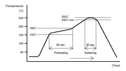
Note 1: Up to 2 cycles of Reflow soldering are possible under the same conditions, provided that there is a return to normal temperature between the first and second cycle.
