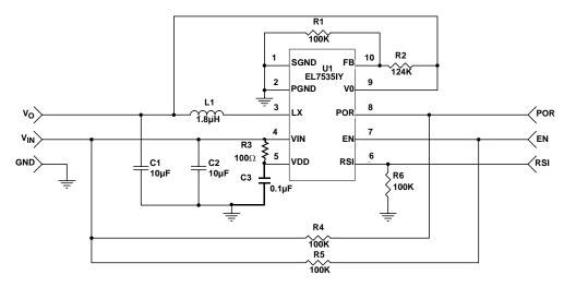
FIGURE 1. DEMO BOARD SCHEMATIC
