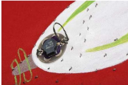
Flip over the circuit to the back side. You can see the two traces between the LEDs and pins 5 and 6, which will need to be crossed. Cut a piece of felt or another thick fabric, or create an alternative bridge if you prefer- you just need something that will insulate between this trace and the previous ones.
