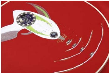
Stitch down the positive side of the last LED and connect it to pin 11.
