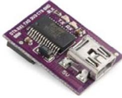
This board serves three separate purposes. First of all, it can **power** the LilyPad Arduino Simple. A power source for your project is one of the most important decisions you'll make. The FTDI Basic will source power from your computer's USB port, and relay it over to the LilyPad Arduino.
