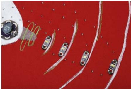
Continue this trace down and around to the negative pin of the Arduino. I neglected to get a picture of this connection, but just be careful not to touch the other traces and to pin it down well with several stitches. Next, cut and knot your thread, and get ready for the final trace! Sew down the positive pin on the buzzer.
