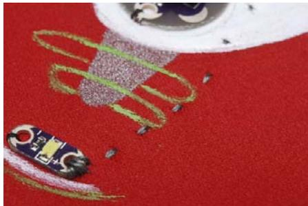
Sew from that positive hole to pin 5 of the Arduino board. You'll want to skirt around the buzzer a little ways, to leave room for the negative trace to leave the buzzer. When you get to pin 5, stitch it down several times before knotting and cutting your thread.
