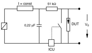
DUT device under test ICU ignition control unit (sensitivity 10 ... 30 μA) Discharge current 10 ... 20 mA
