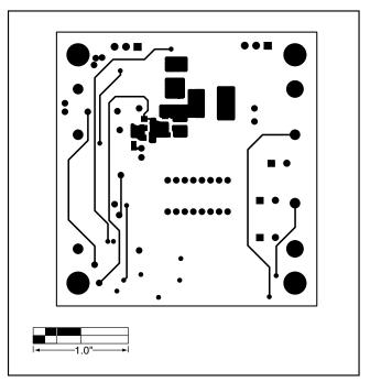
Figure 9. MAX5015 EV Kit PCB Layout—Solder Side
