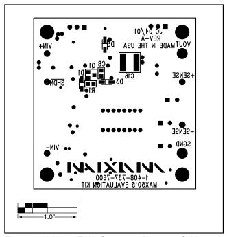
Figure 10. MAX5015 EV Kit Component Placement Guide—Solder Side
