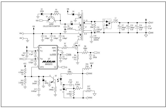
Figure 4. MAX5015 EV Kit Schematic
