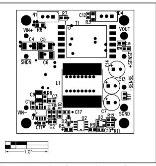
Figure 5. MAX5015 EV Kit Component Placement Guide—Component Side
