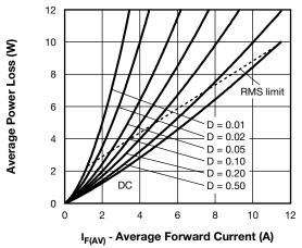
Fig. 6 - Forward Power Loss Characteristics
