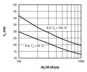
Fig. 7 - Typical Reverse Recovery Time vs.  $dI_{\text{F}}/dt$
