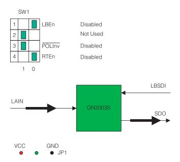
Connector Compensation Disabled. Note: Connection to GND is not allowed.
