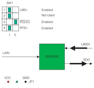
Connector Compensation Disabled. Note: Connection to GND is not allowed.
