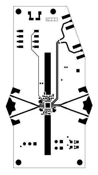
Figure 2-3: XBN2003 PCB Layout — Top Comp.
