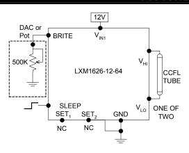
Figure 1 – Brightness Control (Output current set to maximum)
