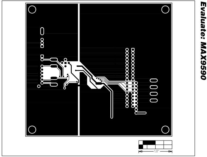
Figure 5. MAX9590 EV Kit PC Board Layout—Solder Side
