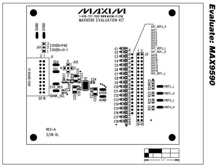
Figure 3. MAX9590 EV Kit Component Placement Guide—Component Side
