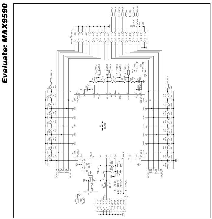
Figure 2. MAX9590 EV Kit Schematic
