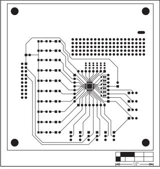
Figure 11. MAX6889 EV Kit PC Board Layout—Component Side
