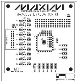
Figure 10. MAX6889 EV Kit Component Placement Guide— Component Side
