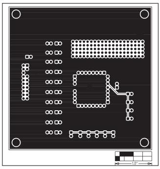
Figure 12. MAX6889 EV Kit PC Board Layout—Solder Side
