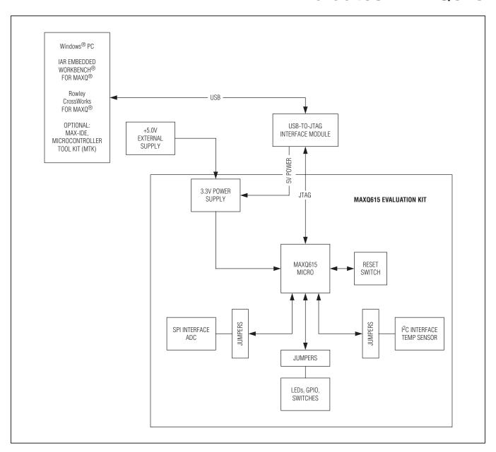
Figure 2. MAXQ615 EV Kit System Block Diagram
