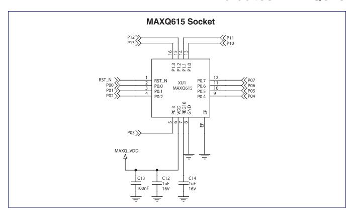
Figure 4. MAXQ615 EV Kit Schematics (Sheet 2 of 2)
